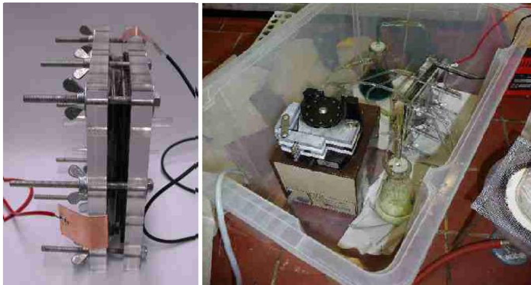
Ill.5.2: Our redox flow cell (left) and the complete setup of the redox flow system
