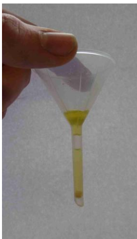
Ill.7.1: zeolite reacts with the acid creating a plug
